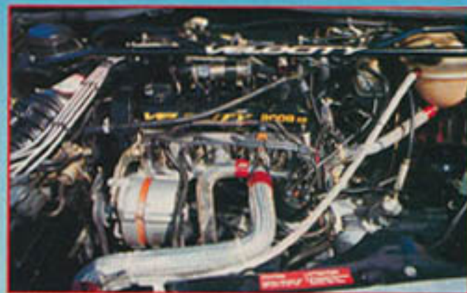
ABOVE - There are quite a few killer performance products languishing within this engine. A R.C. Engineering balanced crankshaft, JE forged pistons, and Neuspeed 268 camshaft, just to name a few.
