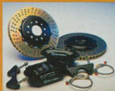
The Mk IV cars are as heavy as they come, and Velocity has developed a brake conversion featuring Brembo and Audi components.
