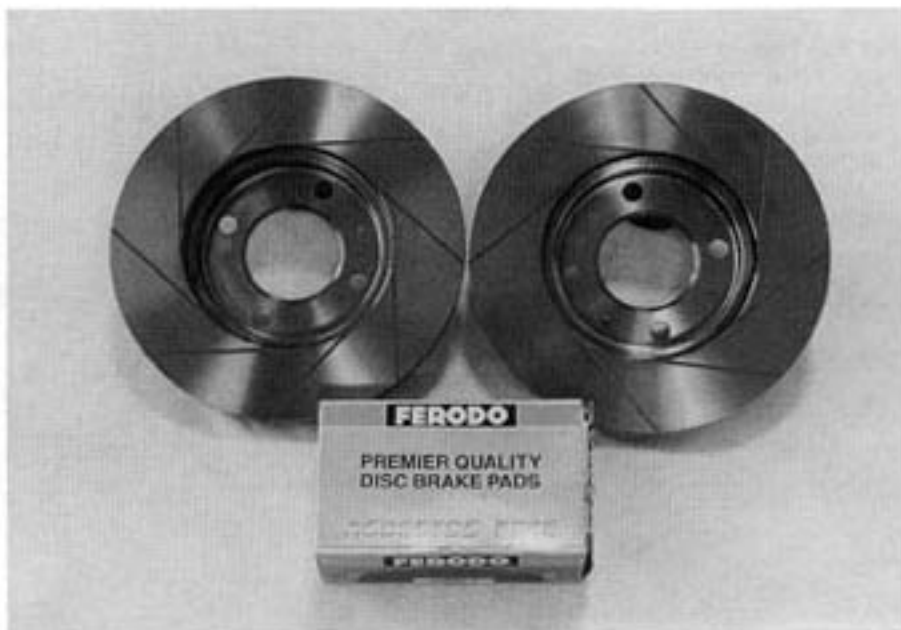
Fig. 4-6. Slotted rotors act similarly to cross-drilled rotors; while less prone to brake fade, they do have a tendency to wear pads quickly.
